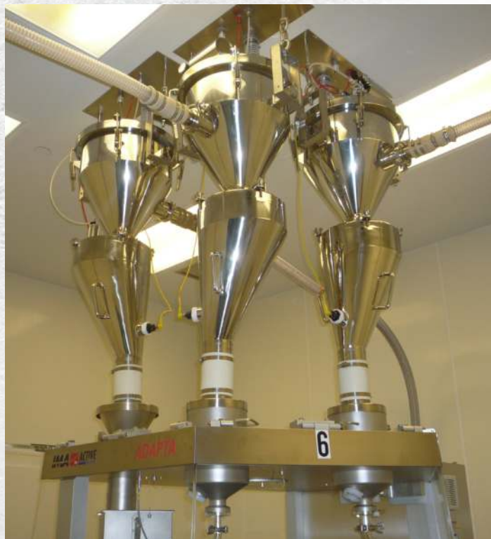
Sanitary vacuum receivers for continuous vacuum conveying of pharmaceutical powders to capsule filling machines, packaging machines, and tablet presses.
