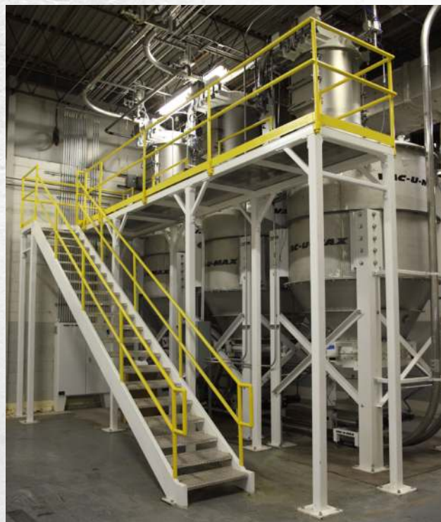
These 300-cu-ft material receivers are part of a pneumatic conveying system that transfers powders in a large-scale candy making process.
