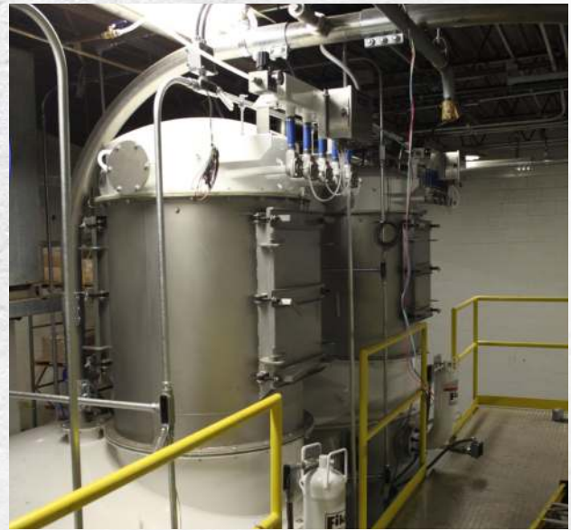
VAC-U-MAX Pulse Dome Filter Covers above VAC-U-MAX Vacuum Receivers equipped with side access doors
